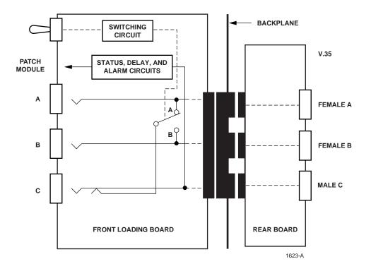
Figure 3-1. Switch Module and Conversion Board
